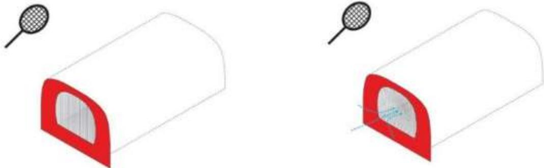
The cable net facade can be compared to a tennis racket. The loads are transferred horizontally and vertically.
